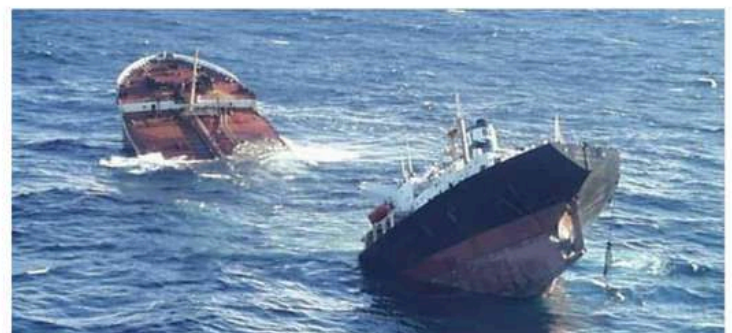
Fig. 1 Structural Failure of the Prestige Tanker
