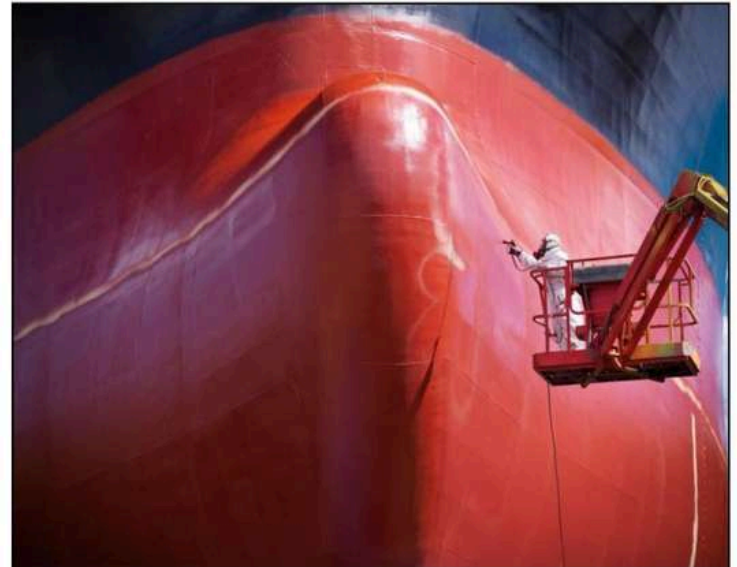
Fig. 3. Hull protection from corrosion
