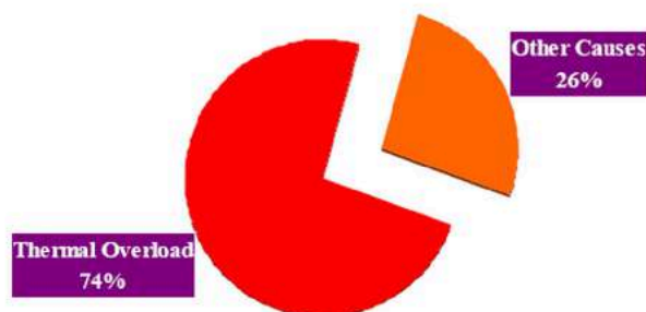
Fig.1: Failure causes of Electronic Equipment
